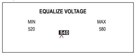
The equalize voltage is also programmable. In the example above, the range is 520 to 580 volts with the default being 540 volts.
